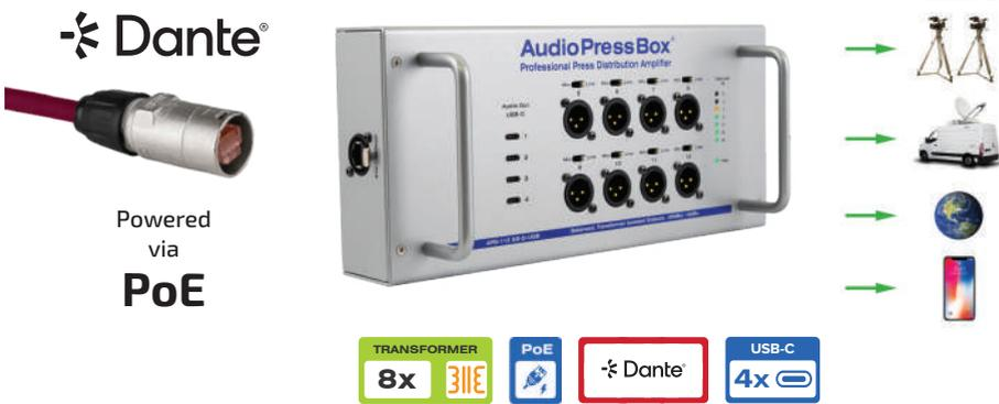
1-channel **DANTE** input, 4 UCB-C outputs, 8 high quality balanced, individually transformer isolated outputs • XLR outputs are switchable between Line or Mic level • The unit is powered only via **PoE** from **DANTE** network, thanks to **DANTE** patching you can easily expand the number of channels or number of outputs by adding other APB-112 SB-D-USBs.
