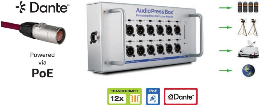
1- channel **DANTE** input, 12 high quality balanced, individually transformer isolated outputs • Each output is switchable between Line or Mic level • The unit is powered only via **PoE** from **DANTE** network, thanks to **DANTE** patching you can easily expand the number of channels or number of outputs by adding other APB-112 SB-Ds.
